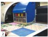
Kornit Digital Allegro directly prints on the fabric using no water at all
