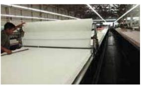
In case of automatic spreading, the number of workers required to handle the fabric reduces to one
